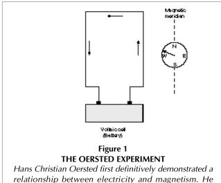
relationship between electricity and magnetism. He showed that a magnetic compass needle, placed near a current-carrying wire, will turn in the direction of the wire.
