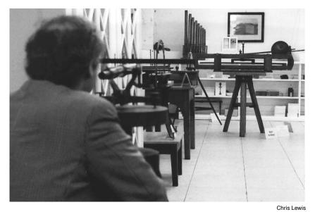
Jonathan Tennenbaum observing the ultra-sensitive receiving apparatus of the Gauss-Weber telegraph, set up here to detect very weak magnetic forces. The telegraph, the world's first, was constructed in 1833, and ran from the Göttingen Observatory to the Physics Building.
