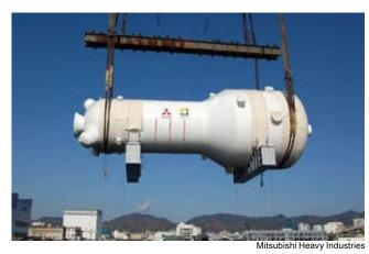
A nuclear steam generator in transport. Mitsubishi delivered two replacement steam generators for the San Onofre nuclear plant in California in February, each weiging 580 metric tons and housing about 10,000 heat transfer tubes.
