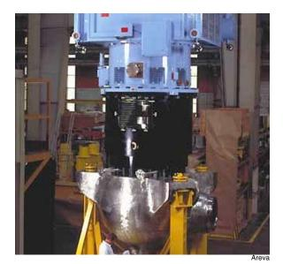
A reactor coolant pump on the production line at France's Jeumont Plant. Each plant requires 70-100 pumps, which will require factories for mass production.
