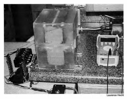
A Seebeck calorimeter which generates a thermoelectric voltage, produced by the temperature difference across a thermal barrier containing thermocouples. This array was built by Dr. Storms.
