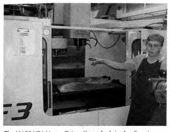
The HASS VF4 Vector Drive. If you look in the direction our guide is pointing, you'll see the bit that is used in a program to fix up the sheet of metal in the photo. The tentacles dangling to the right of the main bit piece are nozzles that spray water to help cool and lubricate the piece being drilled. Another 20 bits for the machine are in storage.
