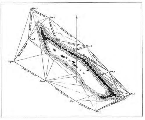
Wilkes's diagram showing the method he used to conduct a running survey of a coral island in the South Pacific. The survey, of the 7-mile-long island, Wilkes wrote in his Narrative on the Ex.Ex., "was performed in 3 hours and 35 minutes."
