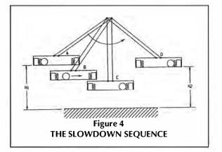
off" delay relay (Photo C). The sweep hand of the timer will continue advancing as long as the pendulum is within the 44- to 48-degree range. Trials indicated that the elapsed time for the pendulum to slow from a zenith angle of 48 degrees to 44 degrees, because of frictional losses, was consistently 9.2 seconds.
