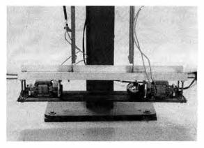
**B** The push-plates of the solenoids are magnetized.
