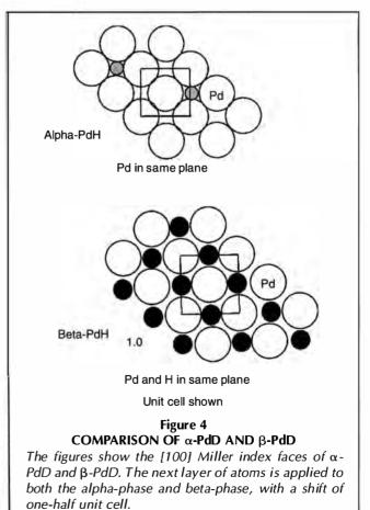
mined by comparing the expected lattice volume, based on the composition, to the measured volume.[114] In forming the  $\beta$ -phase, atoms of Pd shift to allow D atoms into equivalent positions, as shown in Figure 4. Hydrogen lies in the plane, forcing Pd atoms further apart, and occupying the so-called octahedral position. These positions can be filled or empty in a random manner up to a completely filled lattice at PdH<sub>1.0</sub>.
