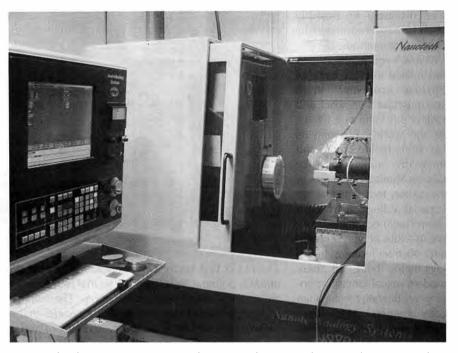
Nanotechnology System's Nano-Lathe. It can shave metal to specifications as close as 1,000,000th of a millimeter.
