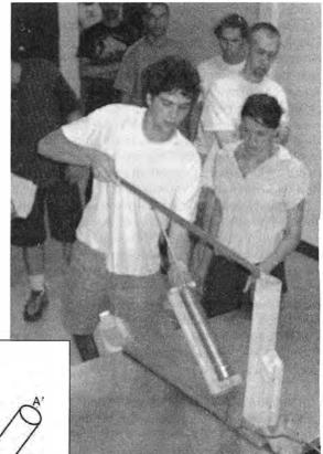
Will Mederski and Rachel Brown demonstrate a steam-driven piston lifting a gallon jug of water. Steam comes from a pressure cooker (not visible).
