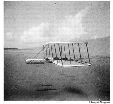
Wilbur Wright lying on the 1902 glider, just after landing. Its skid marks are visible behind. The skid marks in the foreground are from a previous landing.
