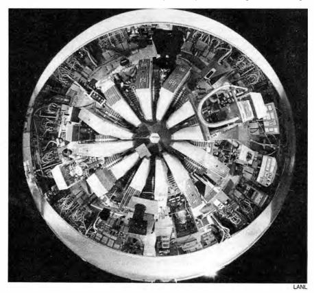
The ZT-40, a reversed field zeta pinch fusion device at Los Alamos National Laboratory. This is another line of promising fusion research that was stopped by lack of funding, although it had already been demonstrated that the concept could work. Other smaller reversed field pinch experiments around the world are in progress.
