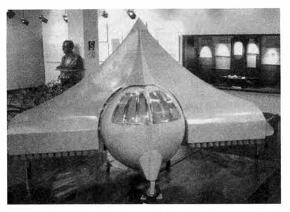
This model of Paulet's Torpedo Plane clearly shows the rocket batteries underneath the spear-shaped triangle, and the ovoidal crew cabin, with windows. The bust of Pedro Paulet can be seen at the top left of the photograph.
