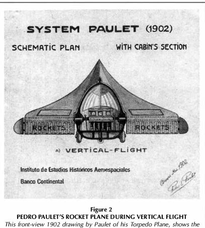
This front-view 1902 drawing by Paulet of his Torpedo Plane, shows the two batteries of rockets, on either side of the crew cabin. When the rocket plane is taking off, and is in vertical flight, the rockets, attached to the spear-shaped frame, are pointed downward.
