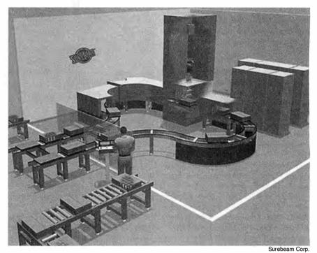
Artist's illustration of an electron-beam irradiation facility. The containerized product travels on a conveyor belt through the e-beam device.
