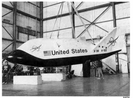
Andy Thomas has proposed that Australia provide a landing site for the Crew Return Vehicle (CRV), that will be developed for the International Space Station. Seen here is the NASA X-38 test vehicle, the precursor to the CRV.
