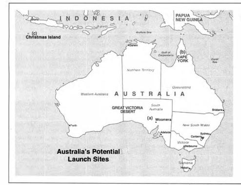
Australia has promising sites to be developed for the launch of commercial satellites. The Woomera test range (a), which dates back to the end of World War II, is ideally suited for testing launch vehicles, which can fly northwest over 2,000 kilometers of virtually uninhabited land, and to put satellites into a polar orbit, launching toward the north.
