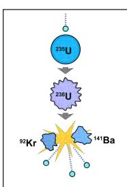
When uranium-235 is bombarded by a neutron, it fissions, or splits apart. Besides its fission fragments, it also releases neutrons, stimulating other uranium atoms to fission, etc., resulting eventually in a self-sustained chain reaction, and a continuous energy source, until so much of fuel has been converted that the reaction is no longer self-sustaining.
