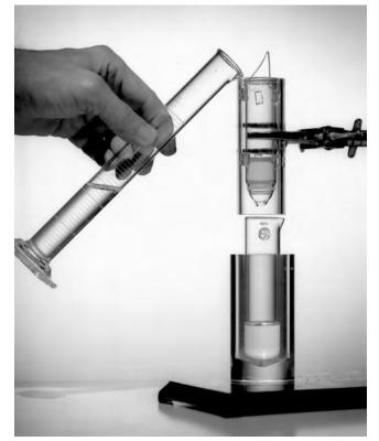
The first chemical separation of technetium-99m from molybdenum-99.
