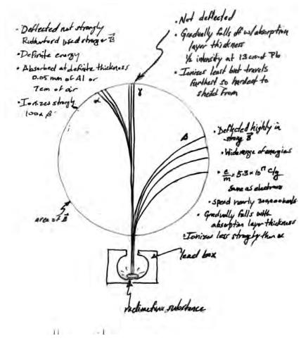
With a strong magnetic field, radiation was able to be split into three different rays with very different properties. They received their names, alpha, beta and gamma, from their different penetration depths. Alpha particles are charged opposite to beta particles, while gamma rays are not charged at all. Alpha particles came out with the same energy, while the energy of beta particles varied widely.
