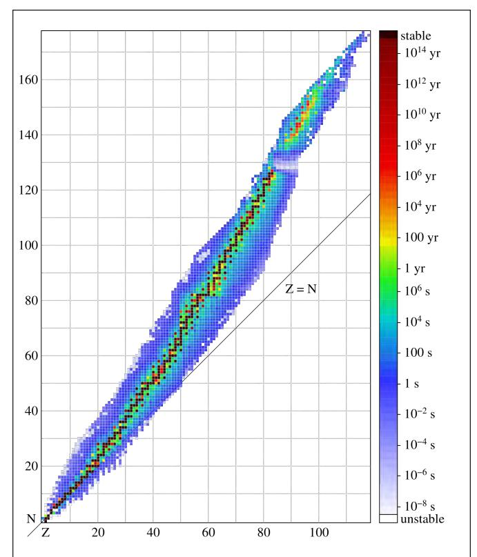
This table of nuclides lists all of the known nuclei. The x-axis represents the number of protons, while the y-axis represents the number of neutrons. Therefore, any column of nuclei represent the isotopes, or variations of the same element. The colors here signify the strength of radiation of each, by indicating the half-life of that particular nuclide, the amount of time it takes for half of any sample to decay. Black indicates stable nuclei.
