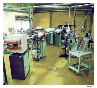
The MGC-20E cyclotron of of Hungary's ATOMKI. Particle accelerators like this one are used to produce the radioisotopes for PET and SPECT imaging.
