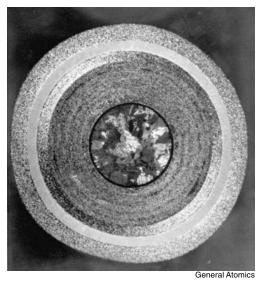
Inside a fuel particle: This is a magnified photograph of a .03-inch fuel particle for an HTR, cut away to show the layers of ceramic materials and graphite surrounding a kernel of uranium oxycarbide fuel. The fission fuel stays intact in its "containment building" up to 2,000°C (3,632°F). This containment makes recycling the fuel more difficult, but not impossible.
