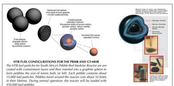
In the General Atomics GT-MHR, the fuel particles are fashioned into cylindrical fuel rods, about two inches long. These fuel rods are then inserted into holes drilled into the hexagonal graphite fuel element blocks, which measure 14 inches wide by 31 inches high. The fuel blocks, which also have helium coolant channels, are then stacked in the reactor core.
