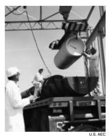
A cylinder of uranium hexafluoride enriched in U-235 is readied for shipment to a conversion facility, where it will be converted to uranium dioxide for use in fuel rods. The cylinder weighs 2.5 tons.
